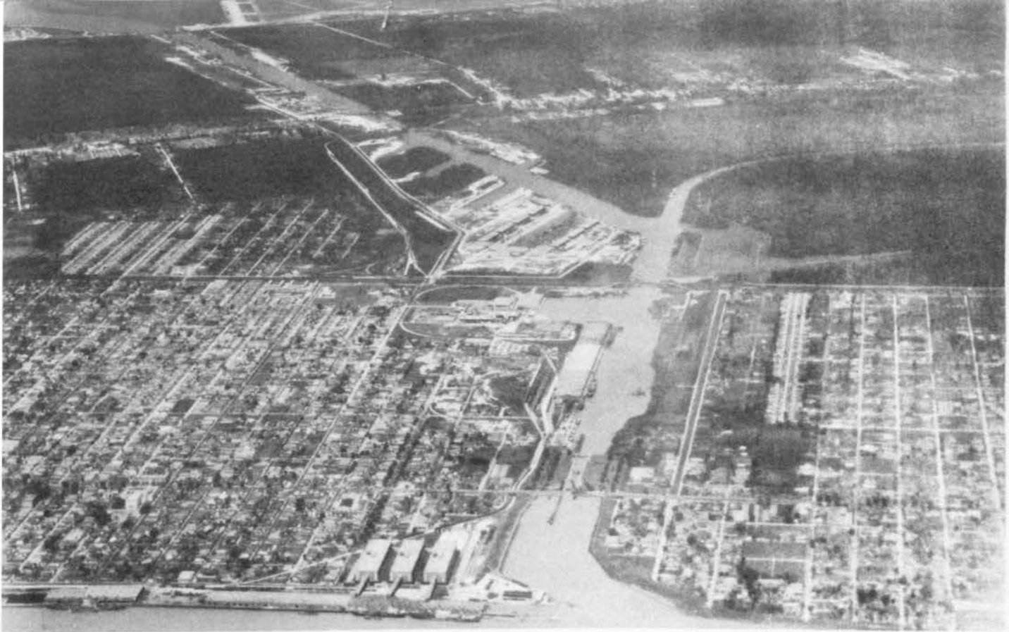
The Industrial Canal, a 5-mile link between Lake Pontchartrain and the Mississippi River at New Orleans, provides wharf space near the business district and space for new industries requiring deep water frontage. The Intracoastal Waterway leads to the right from the Canal.
